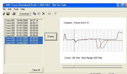
The TDR 510 model allows you to store and export the measurement results and is supplied together with the TDR software.
